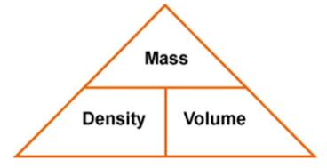
Density (D) =  $\frac{\text{Mass (M)}}{\text{Volume (V)}}$
